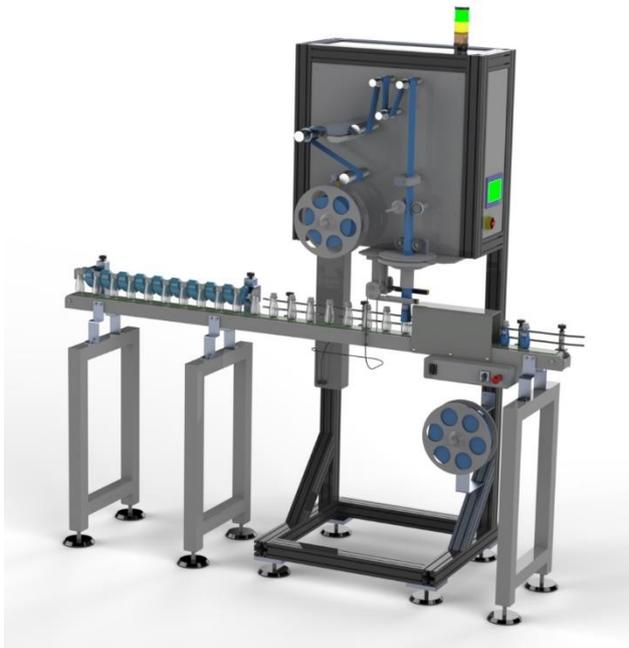
Static electricity may cause the film to stick to the mandrel or, once cut, the sleeve is not properly positioned on the container. Anti static bars or static eliminators are placed at the indicated position to assure a correct functioning of the machine.
