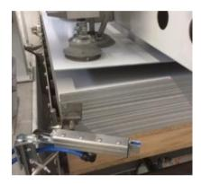
During de-stacking, the single sheet wants to stick to the pile because of static: blowing ionised air between the sheets with (flat-) ionizing air-nozzles or <u>air knives with antistatic bar</u> will solve this problem so only a single static neutral sheet will enter the line.
