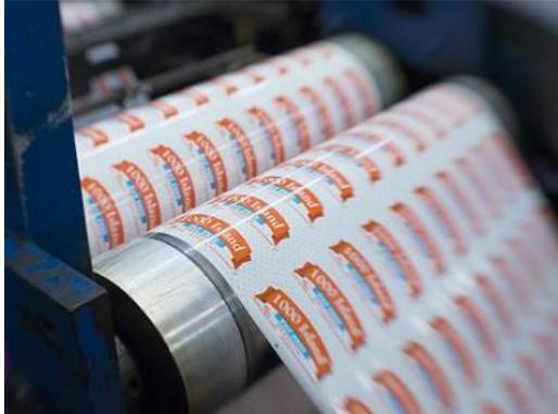
Discharging the web directly after the unwinding process will prevent that an electrostatic charge will attract dust particles from the environment and operators will not experience shocks while passing the web.
