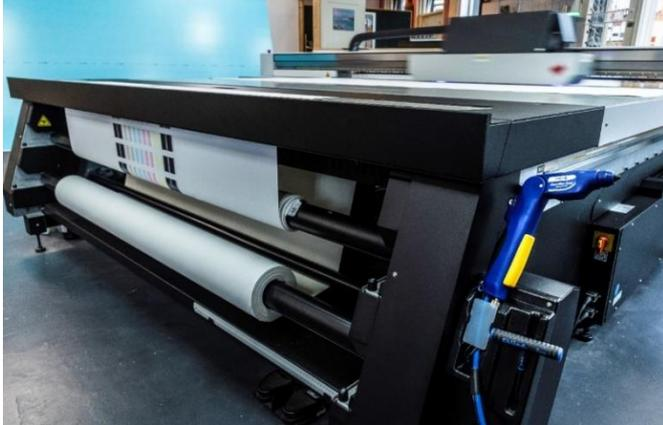
The new [Cleanflex Easy 24V anti static blowgun](#) can be used to neutralise electrostatic charges on the material before printing; f.e. high electrostatic charges (measurable with a [Simco-Ion static meter FMX-004](#)) will occur by removing protective film from plastic sheets.
